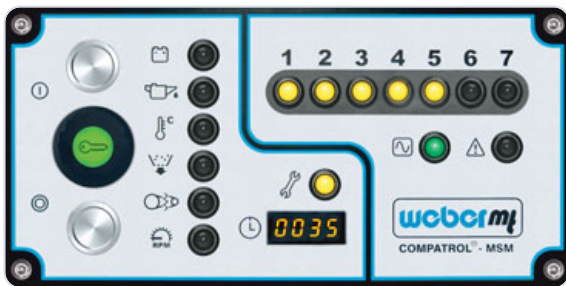
COMPATROL®-MSM notifies: maintenance necessary.
